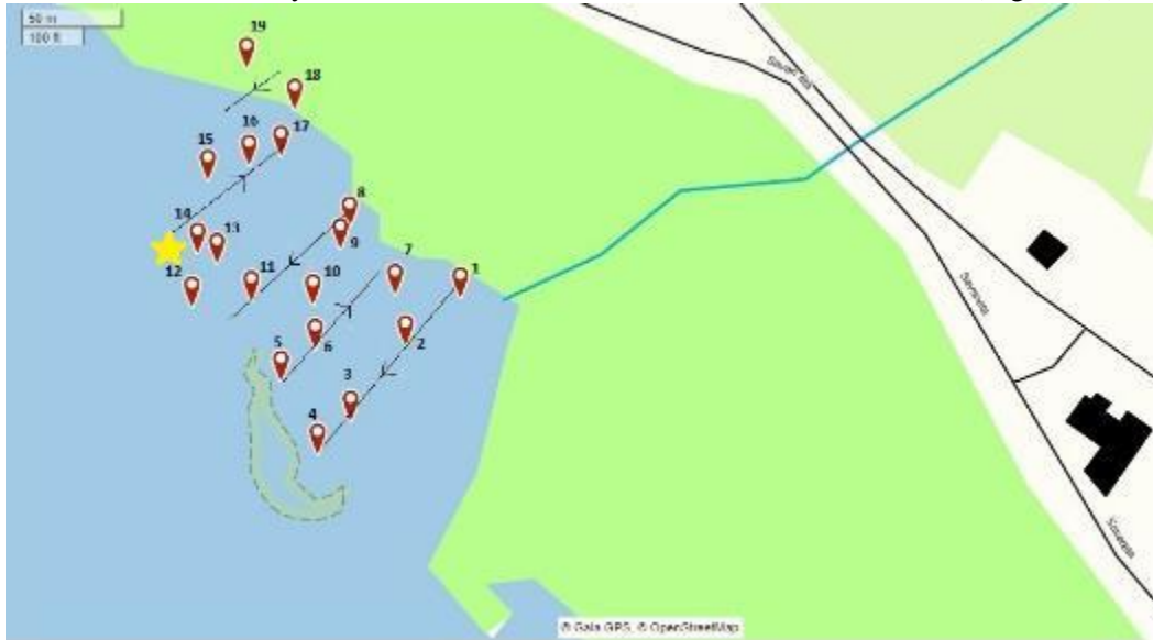
Figure 29. Waypoints indicate stations (N=19, Total replicates=57) at Site 2 Isla di Oro in MP3. Per station, 3 quadrats were haphazardly thrown for field procedures Seagrass-watch 13 . Arrows indicate walking direction. Yellow star designates wave break location on rubble reef.
