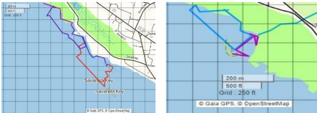
Figure 19. MP3 Site 1 (right) and Site 2 (left) with an overlay grid (1 square: \pm 0.826 \text{ ha}^{-1} ) in Gaia OpenStreetMap. Seagrass extent estimated visually by grid counts; within recorded tracks was \pm 8.43 \text{ ha}^{-1} .
