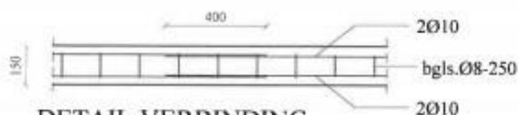
DETAIL VERBINDING OVERLAPPING WAPENING RINGBALK 150MM
