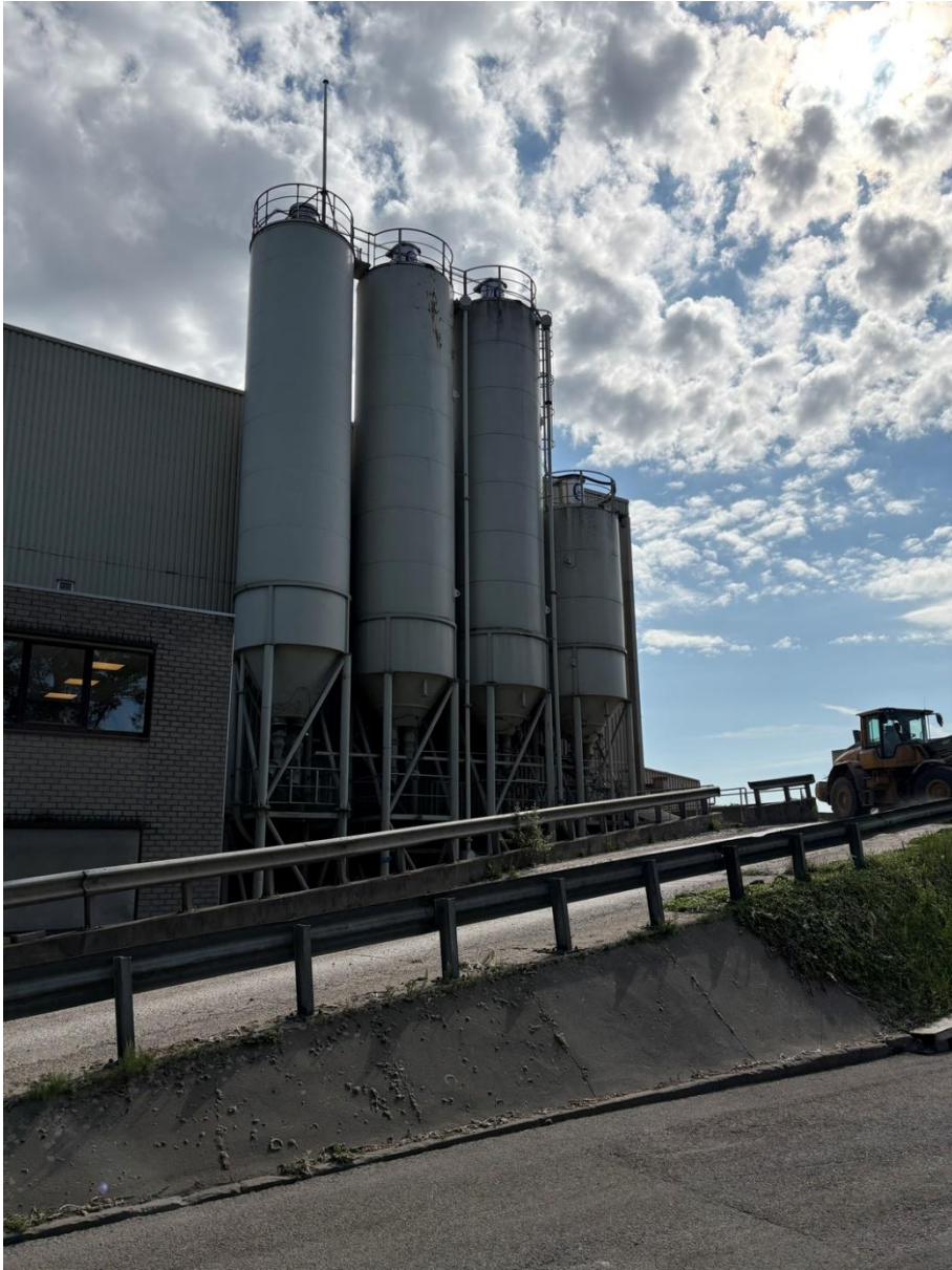
3 silo's of 90m 3 and 1 silo of 40 m 3
