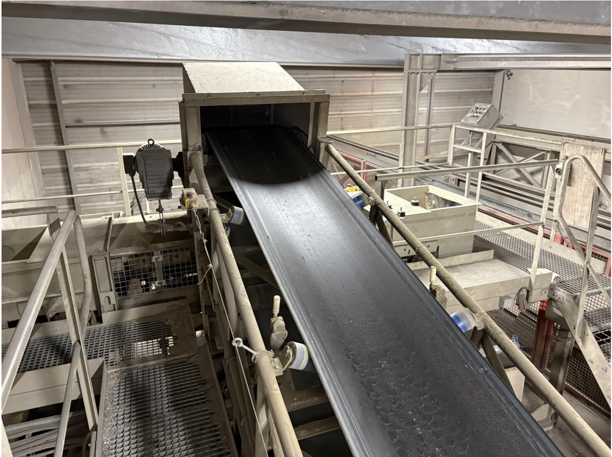
Transport of materials to storage silos with reverseable conveyor
