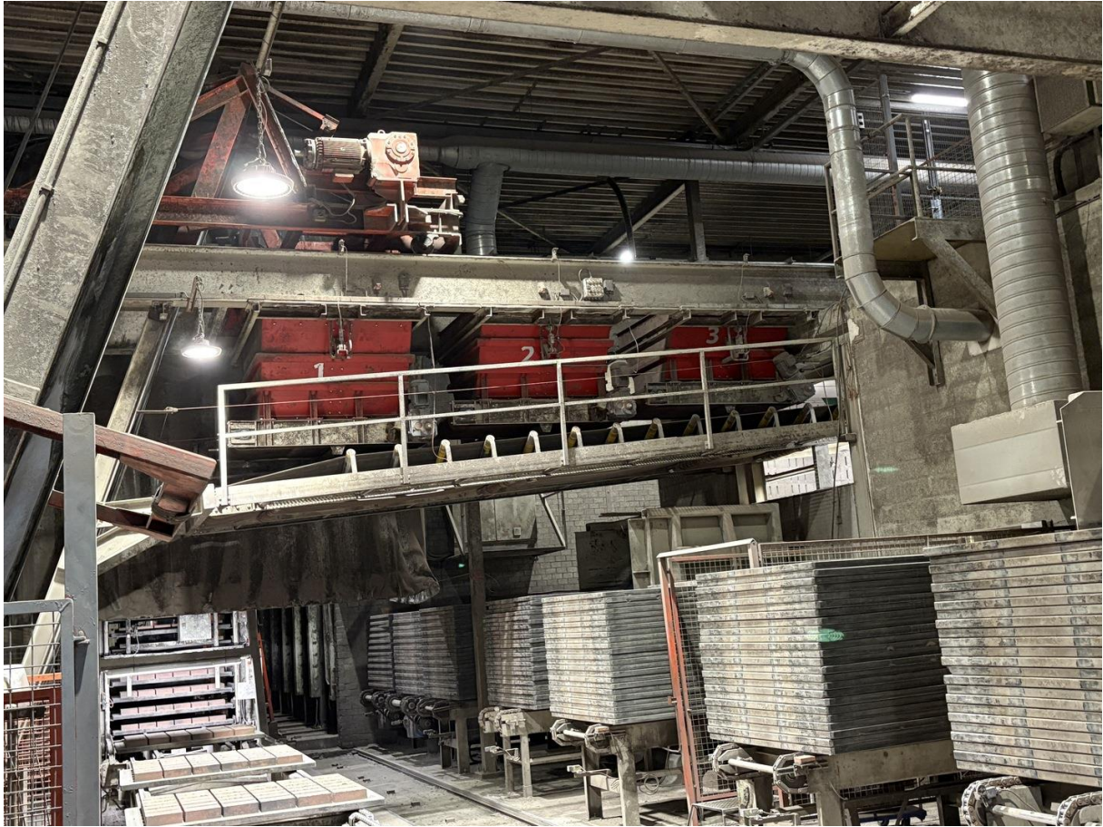
Transport of fresh concrete to machine including 3 color mix hoppers
