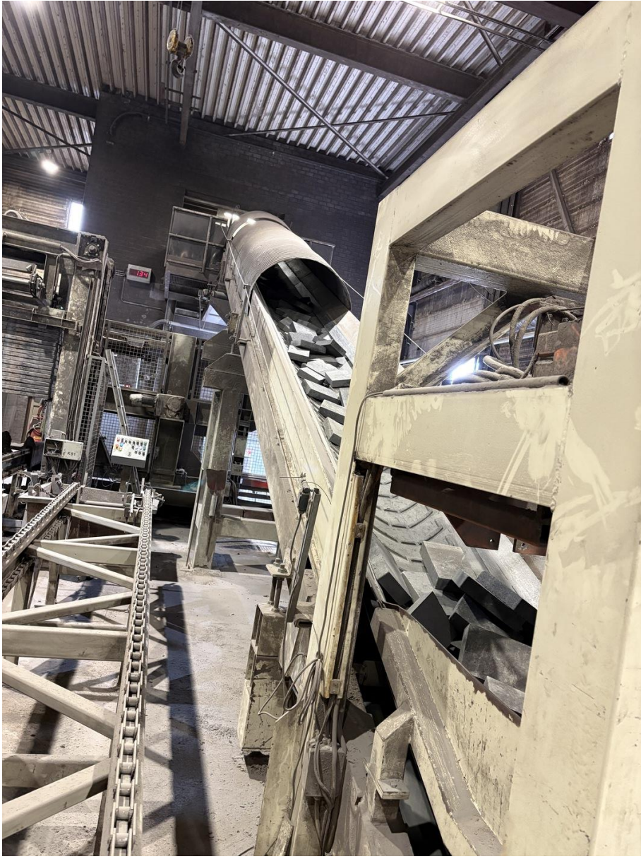
Inline transport of cured products to rumbling plant
