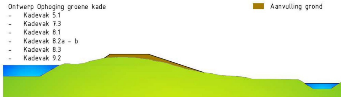
Figuur 8: Principeoplossing ophoging groene dijk Eilandspolder
