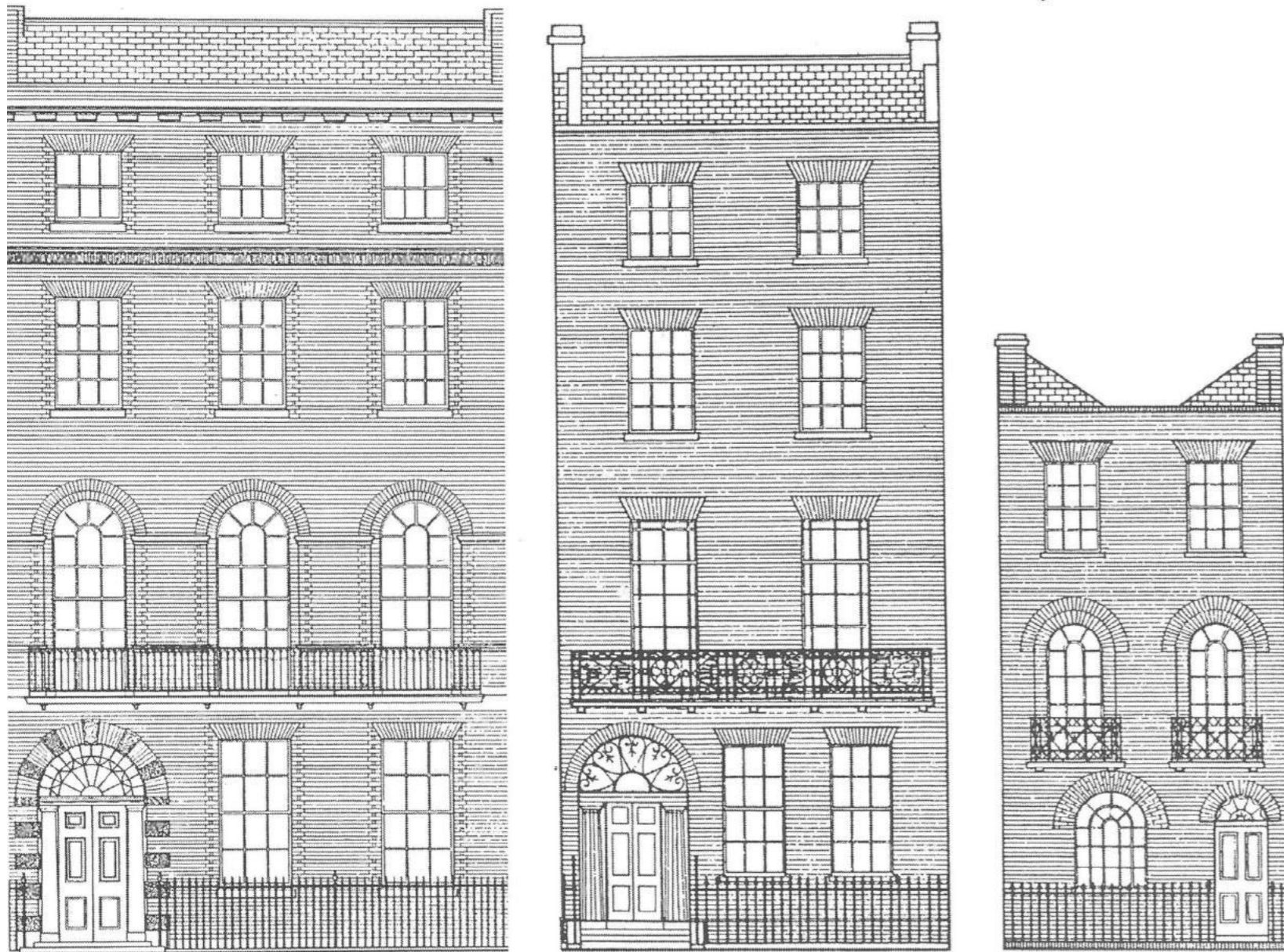
54 'First', 'Second' and 'Third Rate' houses, classified according to floor area and cost, as prescribed in the Building Act of 1774. The First Rate house is from Baker Street, the others are based on examples in R. Elsam's Practical Builder of 1825.
